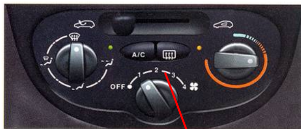
AC / Heater Control Panel
